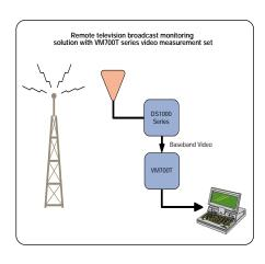
The DS1000 series television demodulator can be part of a total television monitoring system when coupled with a VM700T video measurement set.
